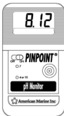
**NOTE:** The pH monitor unit is NOT waterproof and must be operated on a dry surface. Liquid contact on the printed circuit board will cause corrosion and void warranty.
